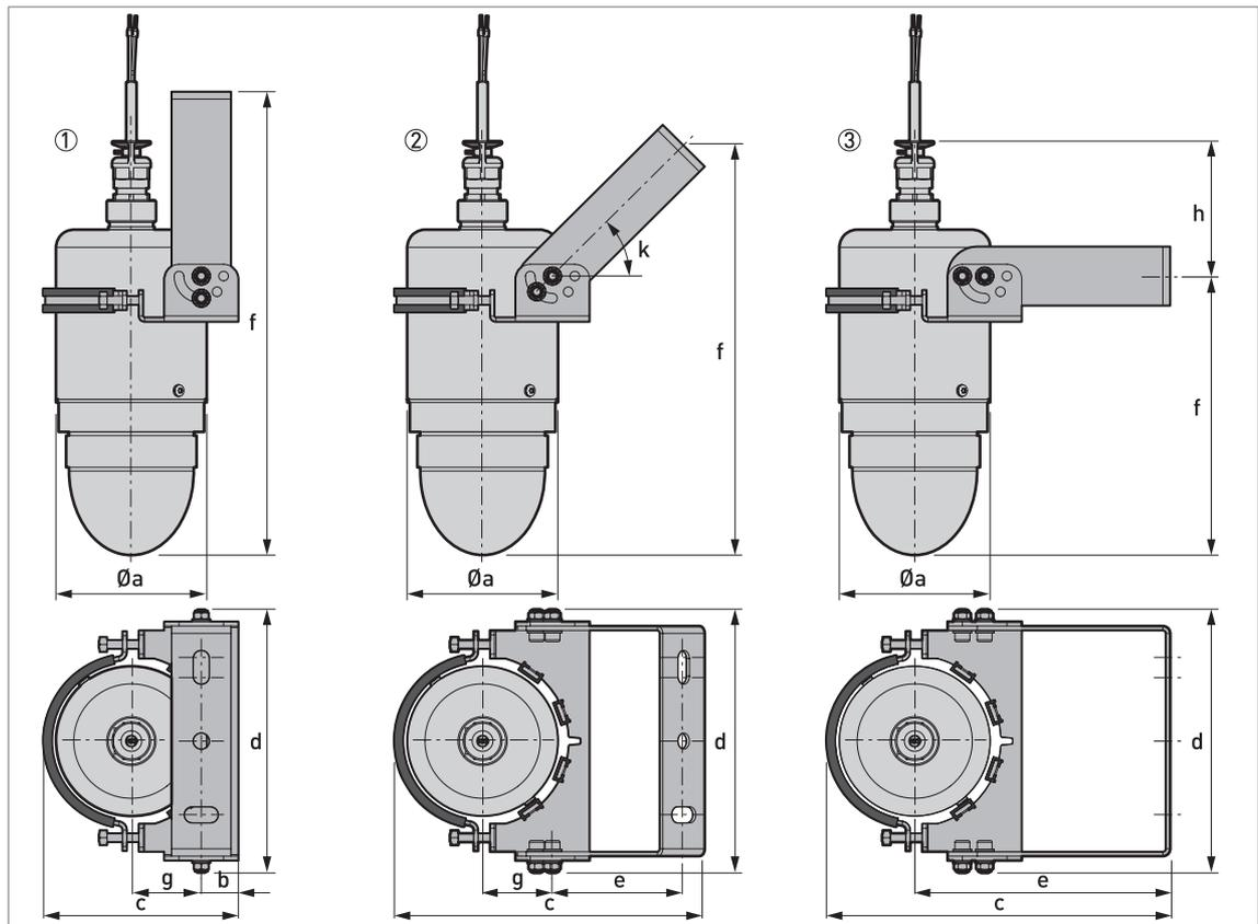
Figure 8-8: Device with orientable collar
