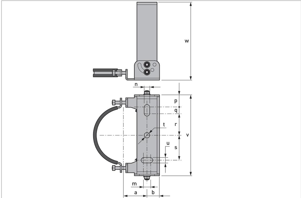
Figure 8-9: Fixed support on the orientable collar
