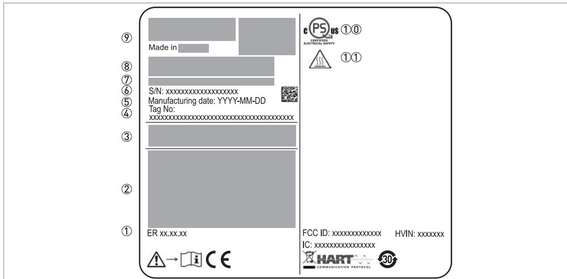
Figure 2-3: Non-Ex nameplate attached to the housing
