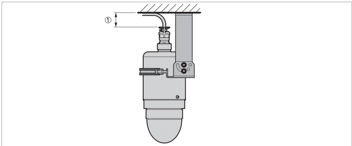
Figure 4-2: Minimum clearance for the electrical cable above the cable gland
