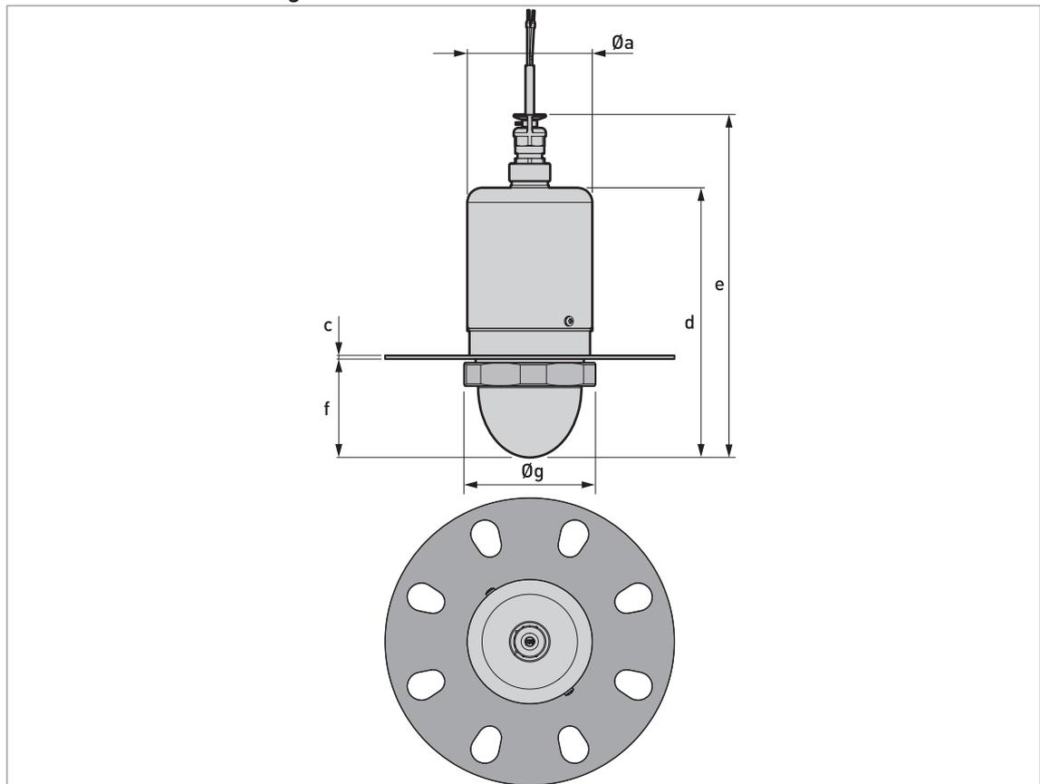
Figure 8-7: Device with bottom flange
