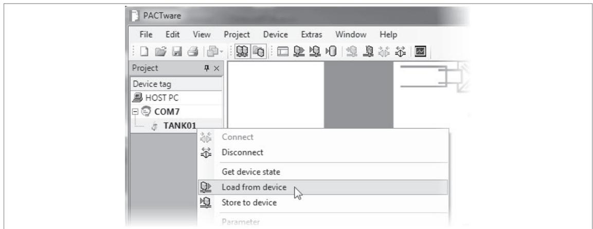
Figure 6-3: Right click on the "OPTIWAVE x400/x500" element in the Project pane (Procedure 3)
