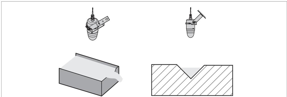
Figure 3-4: Recommended mounting position above a flow channel
