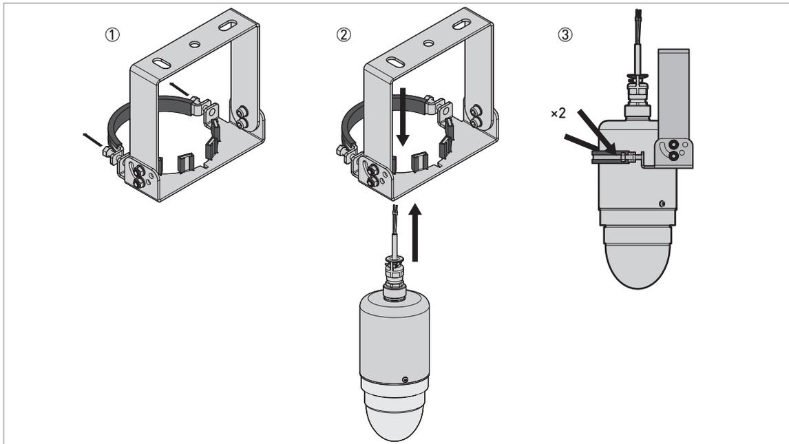
Figure 3-9: How to attach the orientable device collar to the device
