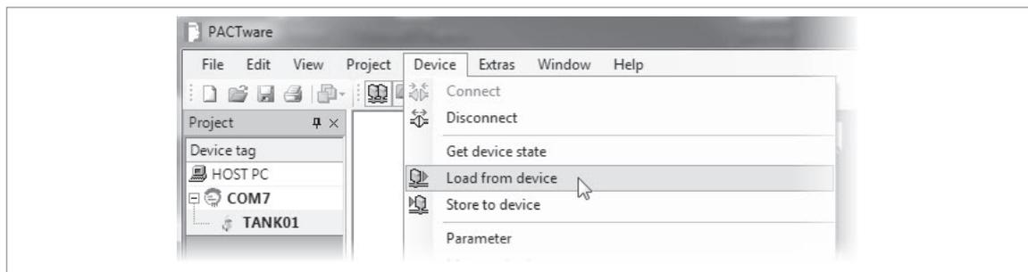
Figure 6-1: Click on "Load from Device" in the Device menu (Procedure 1)
