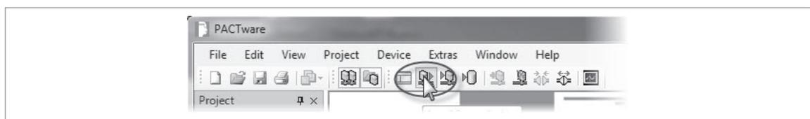
Figure 6-2: Click on the "Load from device" icon in the main toolbar (Procedure 2)
