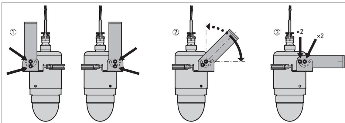
Figure 3-10: How to tilt the orientable device collar to the device
