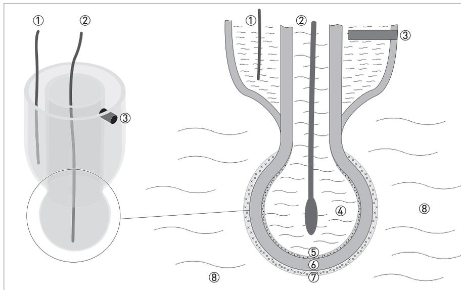
Figure 1-1: Measuring principle for pH measurement
