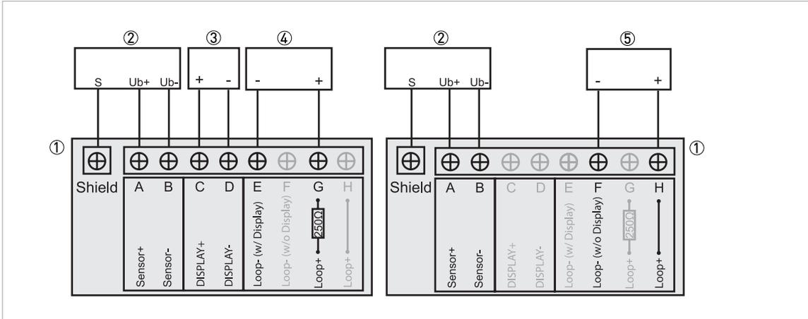
Figure 4-2: Example of a connection with a SJB 200 W-Ex junction box
