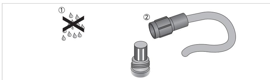
Figure 4-1: Connecting the cable to the sensor
