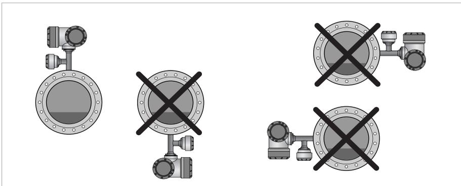
Figure 3-10: Mounting position
