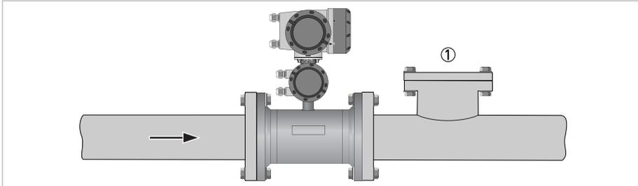
Figure 3-8: Option for cleaning of flow sensor
