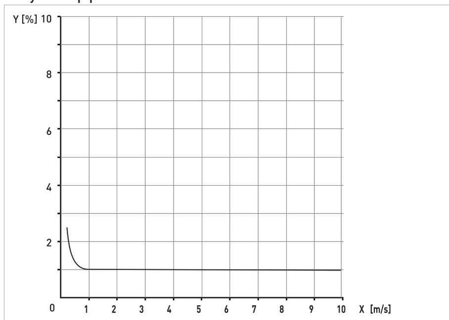
Figure 2-1: Maximum measuring error of measured value
