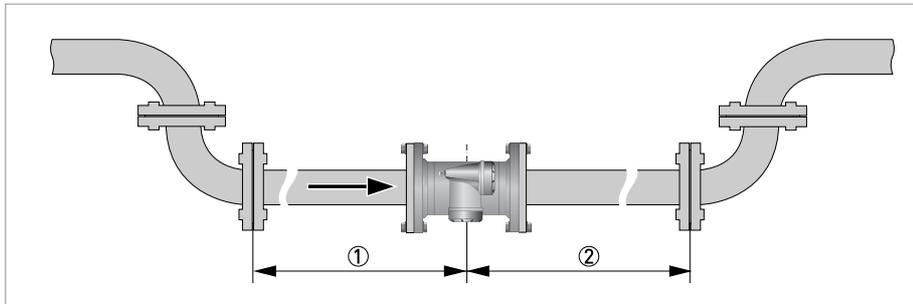
Figure 3-3: Recommended inlet and outlet sections, top view
