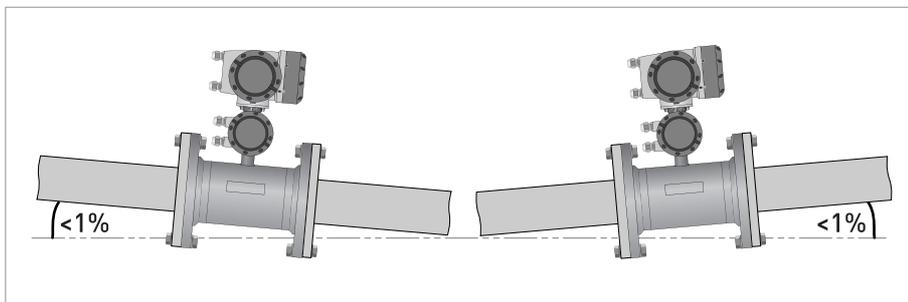
Figure 3-5: Recommended slope
