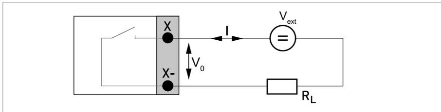
Figure 4-19: Status output / limit switch passive  $S_p$
