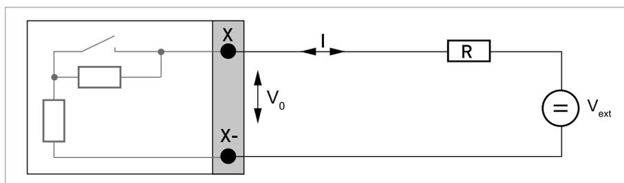
Figure 4-17: Pulse/frequency output passive P<sub>N</sub> according to IEC 60947-5-6 (NAMUR)
