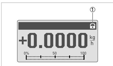
Figure 6-7: Indicator for optical keys in the display
