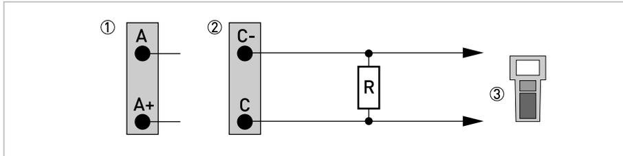
Figure 4-29: HART® connection active ( $I_a$ )
