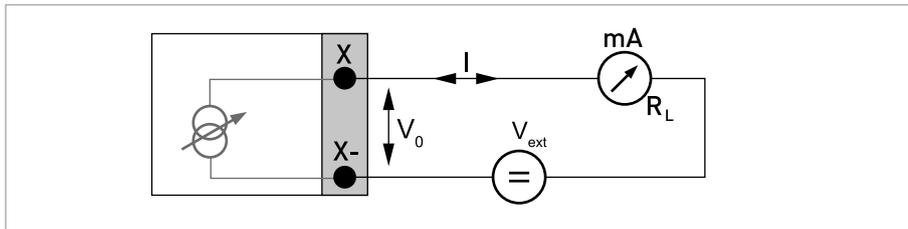
Figure 4-25: Current output passive  $I_p$  Ex i
