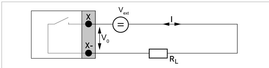
Figure 4-11: Status output / limit switch passive  $S_p$
