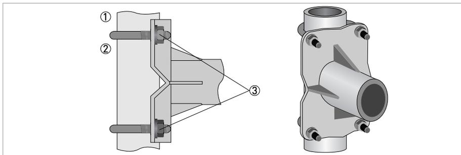
Figure 3-14: Pipe mounting of the field housing
