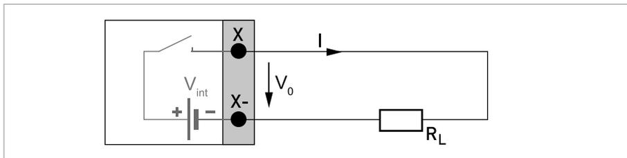
Figure 4-18: Status output / limit switch active  $S_a$
