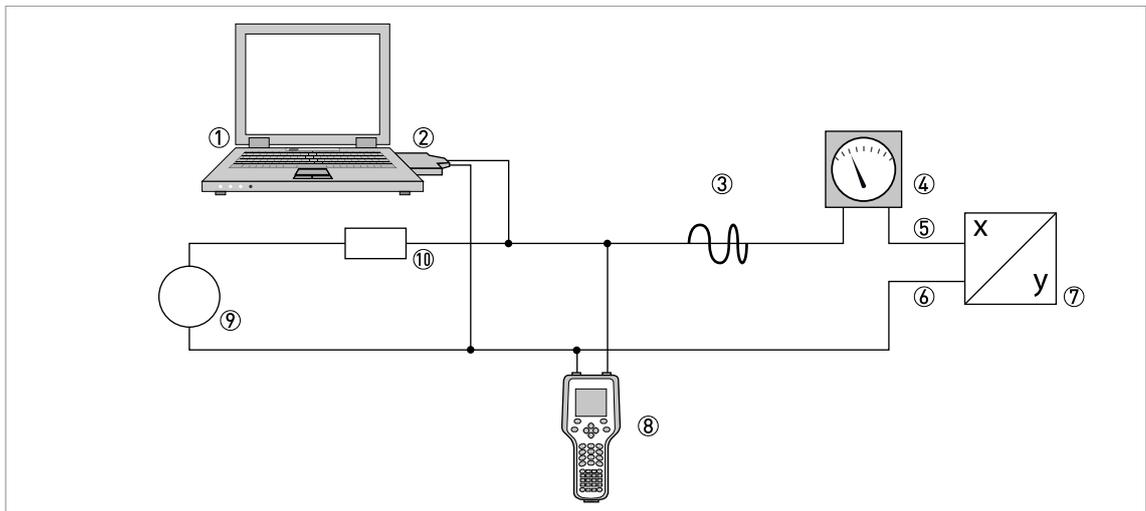
**Figure 9-1: Point-to-Point connection**
