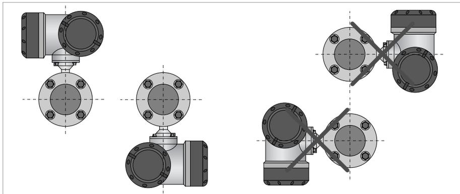
Figure 3-13: Installation position on horizontal pipe sections
