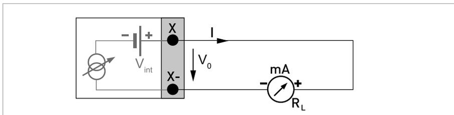
Figure 4-24: Current output active  $I_a$  Ex i
