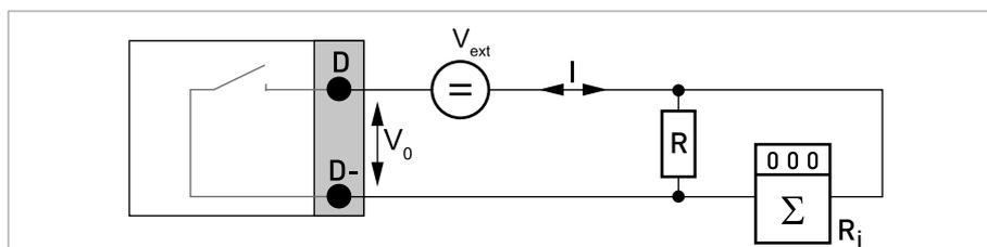
Figure 4-10: Pulse output / frequency output passive  $P_p$
