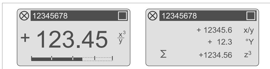
Figure 5-1: Displays in measuring mode (examples for 2 or 3 measured values)
