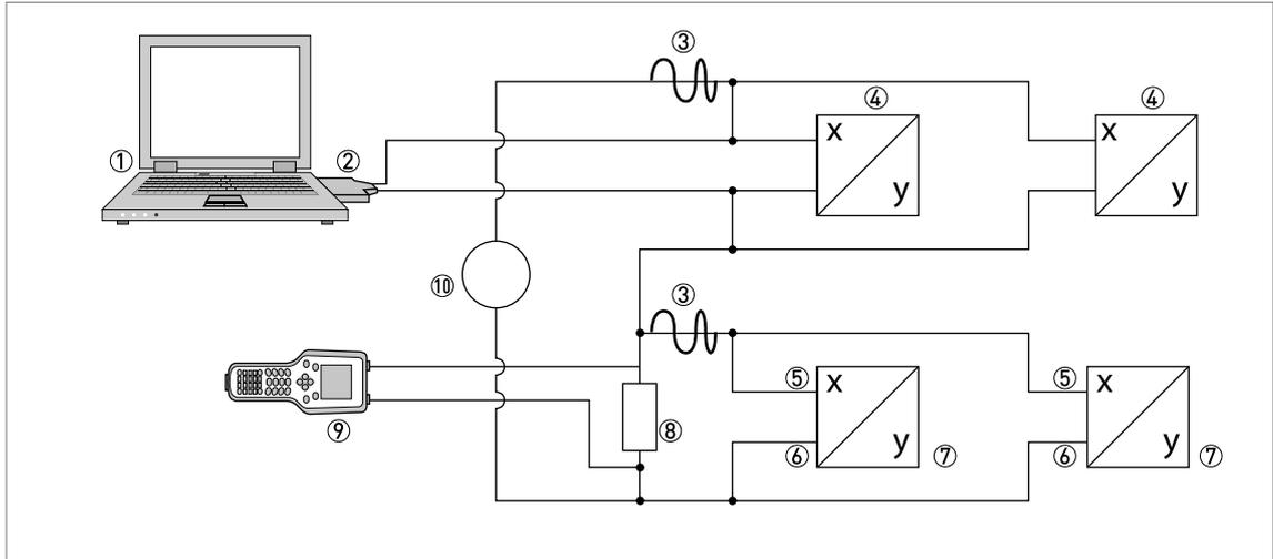
**Figure 9-3: Multi-Drop connection (3-wire connection)**
