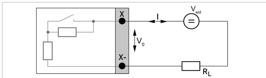
Figure 4-27: Status output / limit switch  $S_N$  according to IEC 60947-5-6 (NAMUR) Ex i
