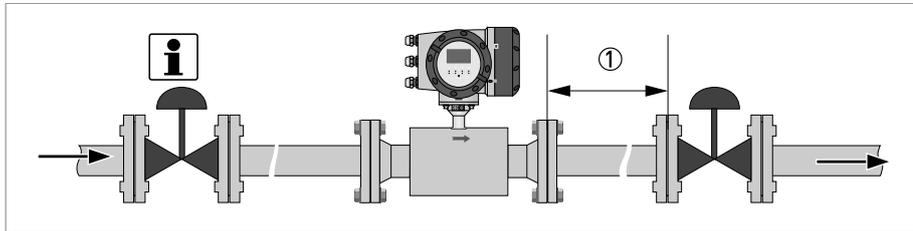
Figure 3-9: Installation in front of a control valve
