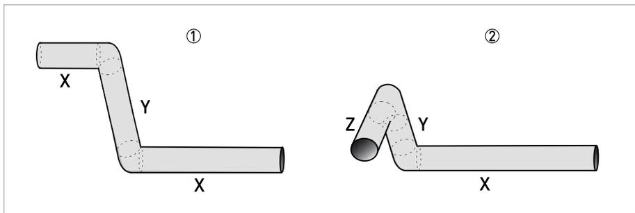
Figure 3-4: 2 and/or 3 dimensional bends upstream of the flowmeter
