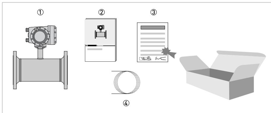
Figure 2-1: Scope of delivery - compact version
