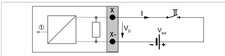
Figure 4-22: Control input passive  $C_p$
