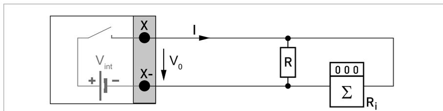
Figure 4-15: Pulse/frequency output active  $P_a$
