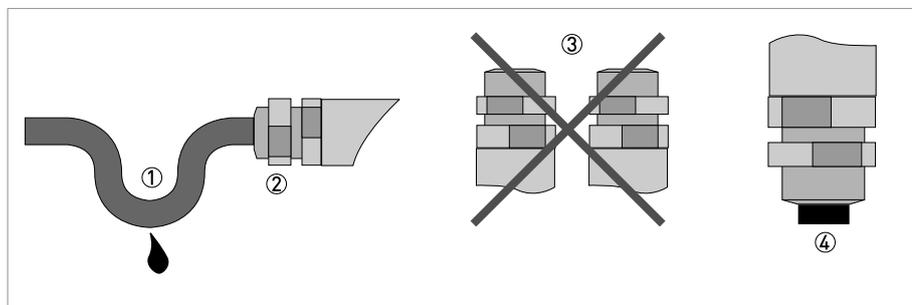
Figure 4-1: Protect housing from dust and water
