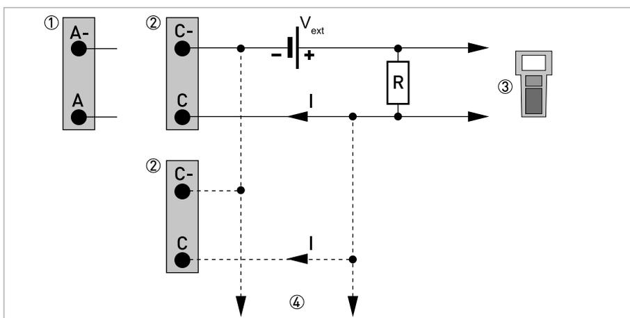
Figure 4-30: HART® connection passive ( $I_p$ )
