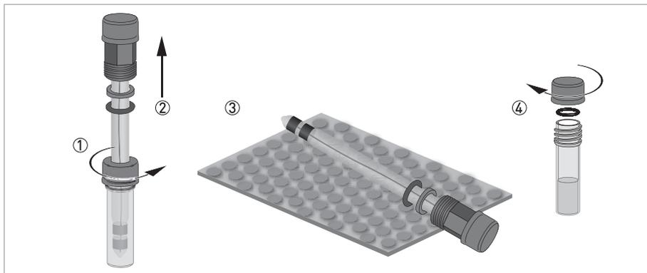
Figure 3-1: Handling the sensor
