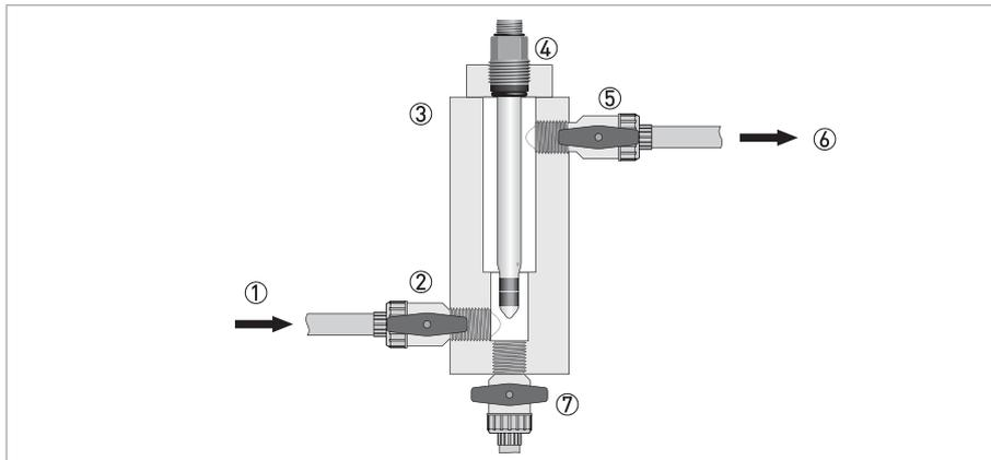
Figure 3-2: Measuring point using the flow cell of the OPTISYS CL 1100 measuring system
