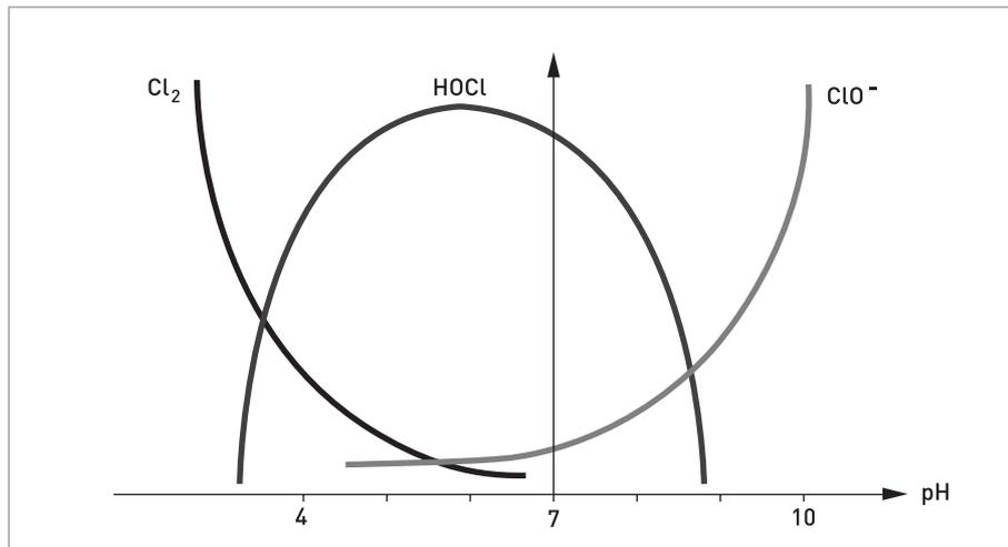
Figure 7-2: Composition of free chlorine depending on pH value
